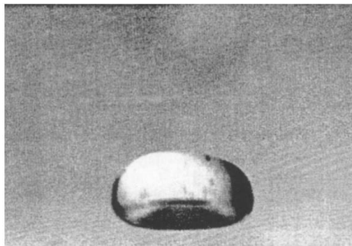
Plate 12. Oscillating water drops of a_0 = 3.5 mm, freely suspended in the vertical air stream of a wind tunnel; observation is taken from below the drop's equator.
