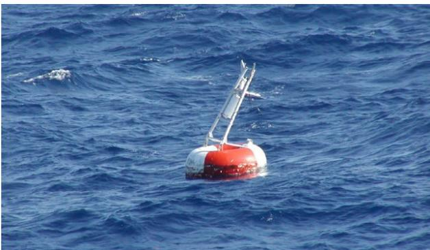
*Damaged TAO buoy, with the superstructure tilting at an angle. Source: B. Burnett, NDBC, 2009 (DBCP-25)*
