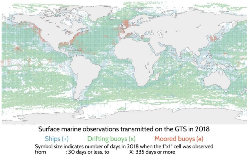
Figure 4: Data coverage by the three major components of the Global Observing System (GOS) (i.e., ships, drifting buoys, and moored buoys) based on information received by Météo-France through the GTS in 2018 (see legend for symbol details). (from *Front. Mar. Sci.*, 30 August 2019 | <https://doi.org/10.3389/fmars.2019.00419> )
