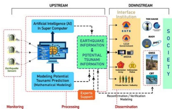
The end-to-end of the Tsunami Early Warning System (InaTEWS)
