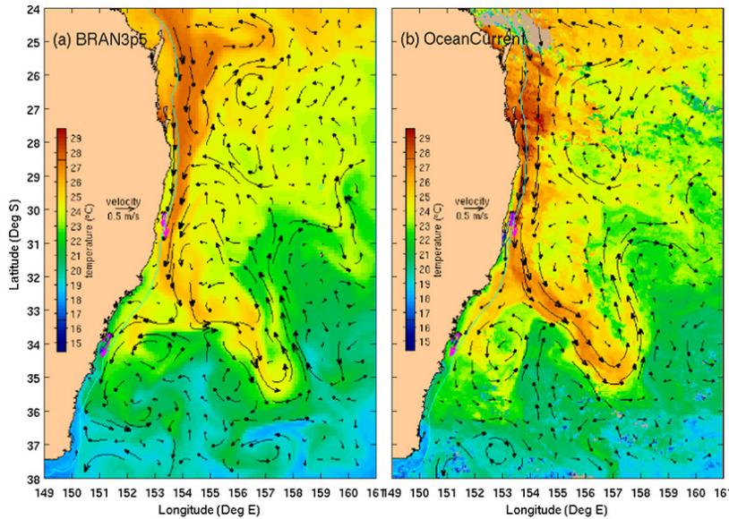
Typical example of (a) Bluelink reanalysis fields and (b) observed fields for the Tasman Sea. Colour shows SST, arrows show surface velocity. (This comparison is adapted from: [www.marine.csiro.au/ofam1/bran1/br3p5\\_EAC\\_tv12/20120111.html](http://www.marine.csiro.au/ofam1/bran1/br3p5_EAC_tv12/20120111.html).)
