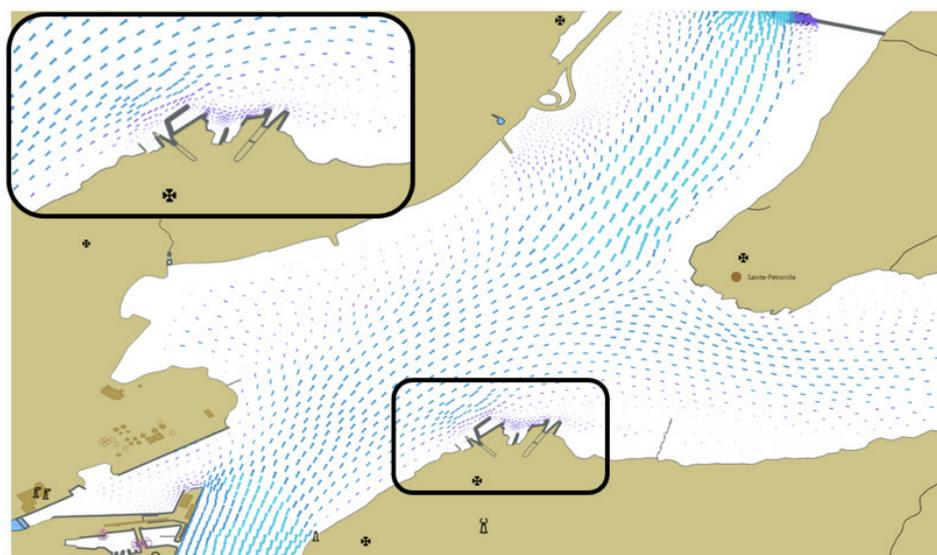
*An example of product for E-Navigation application generated by a high resolution estuarine river 2D prediction system run by the Canadian Meteorology and Environmental Prediction Center H2D2 (Matte et al 2017)*
