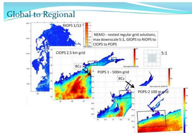
*An example of the prediction systems cascading approach used to generate products and services at high spatial and temporal resolution, for the Bay of Fundy, Canada. (Paquin et al 2019)*
