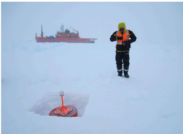
*Expendable remotely-operating instrumentation on, in and below the sea ice, as pictured here, provide crucial information on the state of the sea ice and its snow cover and how it evolves and moves in response to atmospheric and oceanic forcing. (Photo: P. Heil)*
