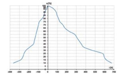
Fig. 1. Example nonparametric design hydrograph obtained by Archer's method
